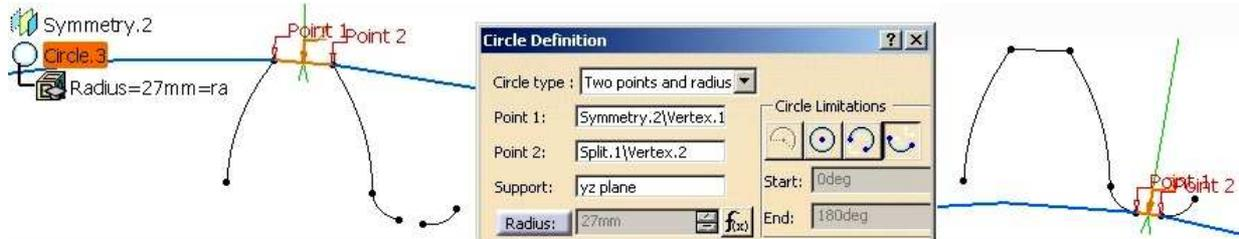
Fig. 2. Completing the tooth profile.
