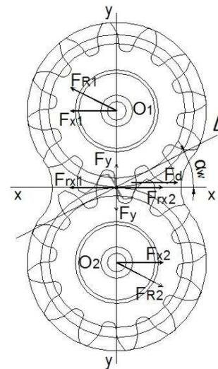
Fig. 7. Tangential and radial forces loaded on gearing and shafts.
