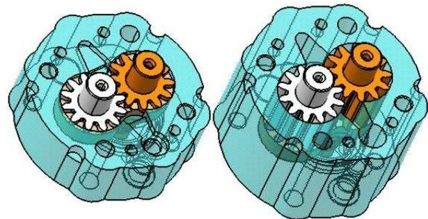
Fig. 5. The pump assembly for min/max flow values.
